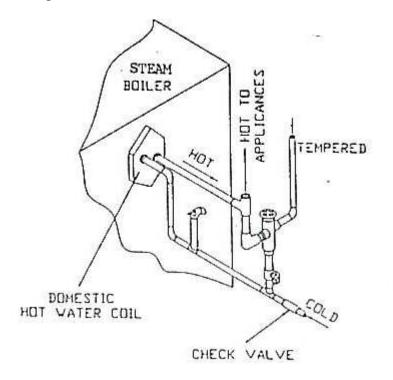
The third method uses a small pump to circulate water continuously between the coil and existing hot water heater. It is also necessary to include a tempering valve on the supply side of the storage tank/water heater.
