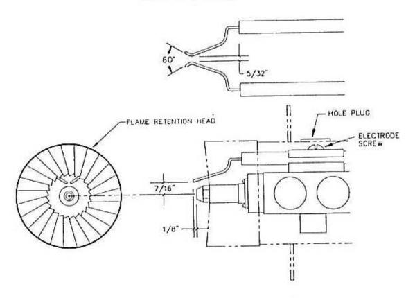
Prior to installing the burner, examine flame retention head and ignition electrode position. This
