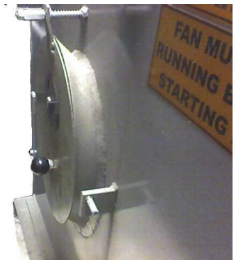
Sight Tube Flap in Closed Position
