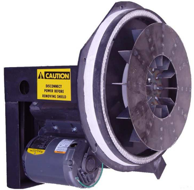
Belt-Driven Fan Assembly Removed from Boiler and Showing White Ceramic Heat Shield
