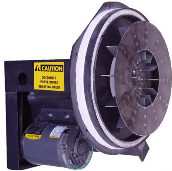
Belt-drive fan assembly removed from boiler and showing white gasket
