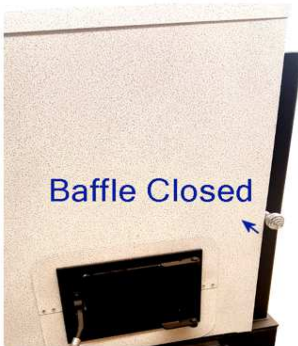
Slide Baffle Closed (Use when draft is good)
