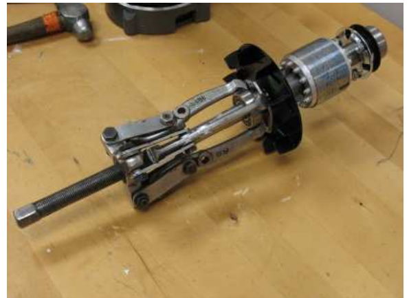
Jaw Puller at the Ready on Motor Bearing
