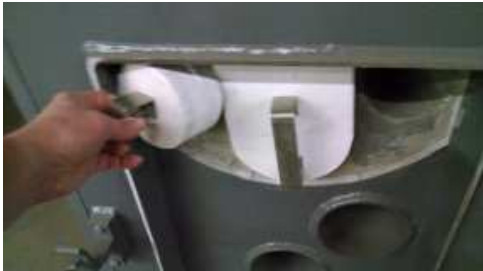
EPA Side Tunnel Plug Install
