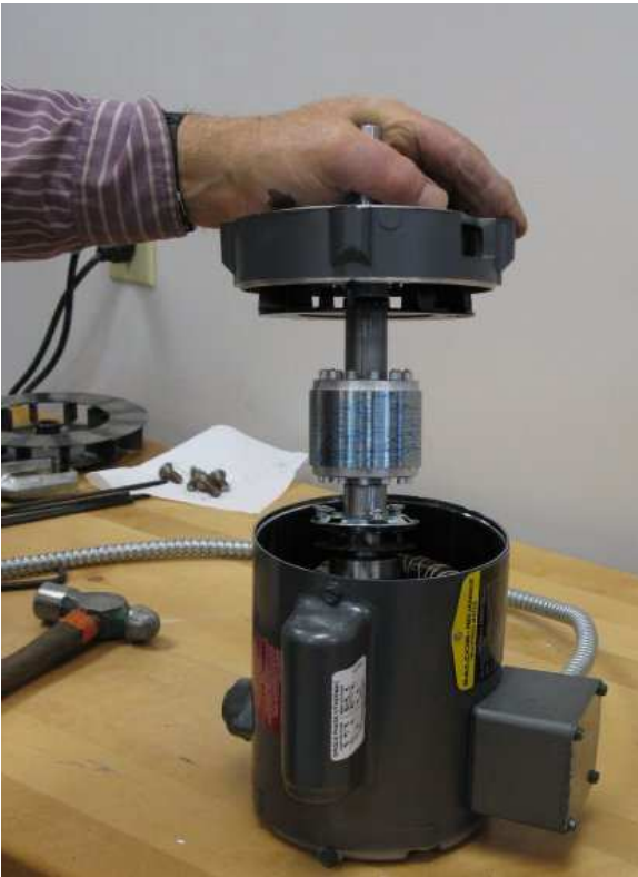
Lifting the End Shield with Armature
