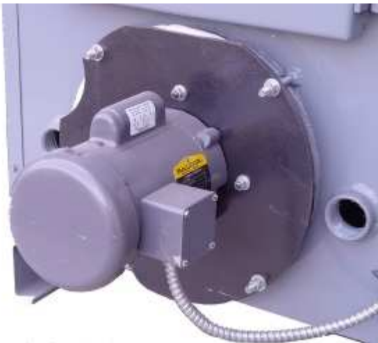
Direct-drive fan attached to boiler
