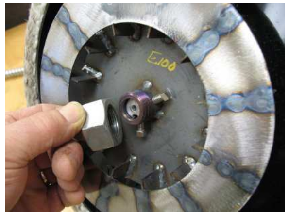
One Inch Nut for Pulling Fan
