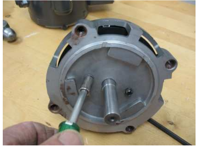
Loosening Screws Securing Bearing to End Shield
