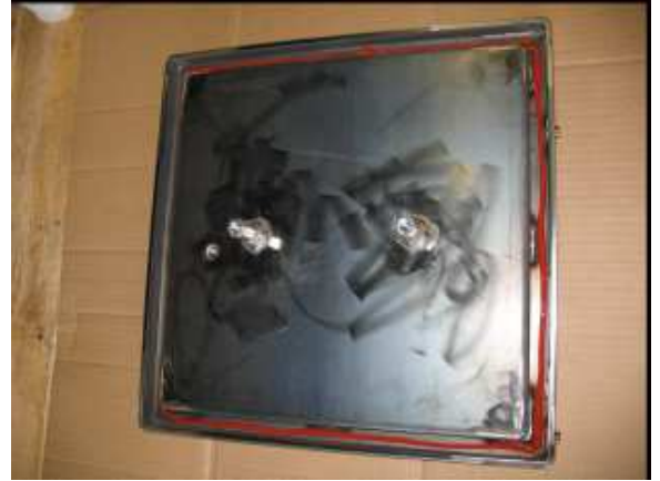
Load Door with Old Seal Removed and High Temperature Silicone
