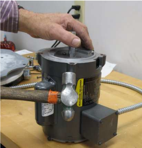
Loosening Motor End Shield from Motor
