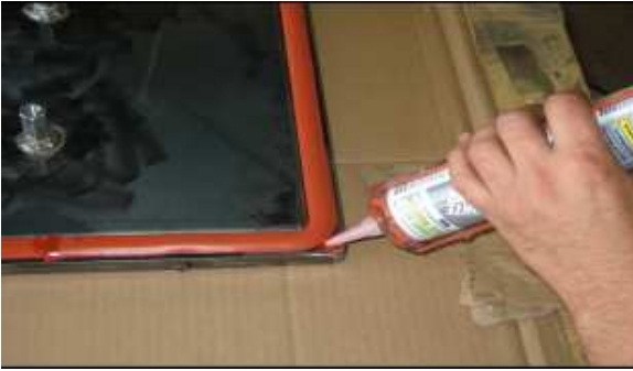
Reinforcing Corners with High Temperature Silicone
